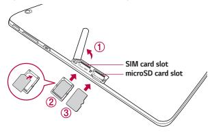
3 If you want to use a memory card, insert the memory card into the slot. Make sure the gold contact area is facing downward. Slide the microSD card into the slot until it "clicks" into place and then close the slot cover.
